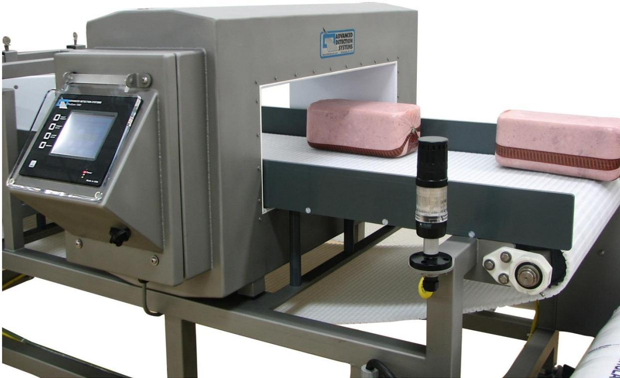
**Product Effect** is a term used to quantify the magnetic and conductive fingerprint of a product for metal detection purposes. All products have a product effect, and metal detectors must factor the magnetic and conductive properties of the product and the environment into the mathematical equation of determining detector sensitivity and detection capability.
